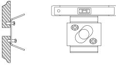
2 Make the connection between the first fix cabling and the luminaire using the IP connectors provided (first fix cabling must be between 22AWG and 14AWG). Insert sheathed cables into the connector and compress using pliers. Do not trap cables when securing the fitting.
