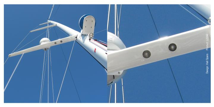
This has been specifically designed for use on yacht spreaders to illuminate the deck or other spreaders below. It is fitted with the latest LED technology and machined from a solid billet of high grade aluminium. This is hard anodised making it resistant to harsh sea environments. The narrow 12 degree beam will light a deck from 9m.
