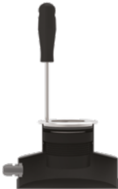
Ring is pulled up and expands the O ring, locking fitting into the housing
