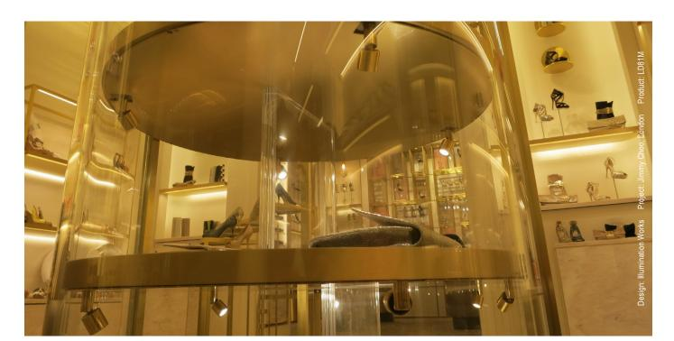
The LD81M is a smaller, more discreet version of the LD81, using the same LED, optics and mounting methods. Maximum output is 1.2W compared to 2.4W in the LD81. Each mounting method is custom made to each projects requirements, allowing the designer to tailor the lighting layout for each display. The best method of specification for these spotlights and mounting systems is to send us a sketch of what is required. This can then be discussed and we will produce a project specification and quote.
