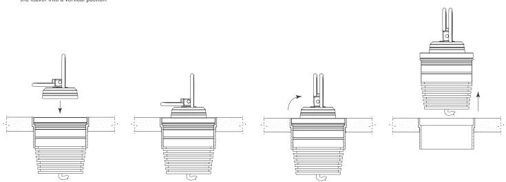
When adjusting or rotating the fitting do not use the HT-154-G hand tool to move in situ. Remove the fitting entirely, realign and then place the fitting back into its fixing option. Note: Rotating the fitting while still in place may result in a comprimised IP seal.
