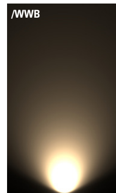
Extra Wide Beam 700mA using a 65° optic
